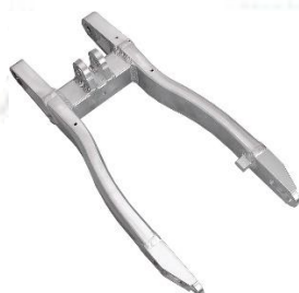
Fig.1 Sand casted Swing Arm
