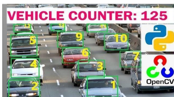
Figure 3: Data extraction (vehicle count) using OpenCV
