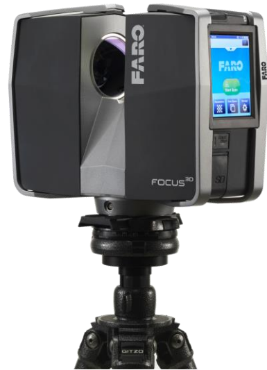
Laser surveying machine
