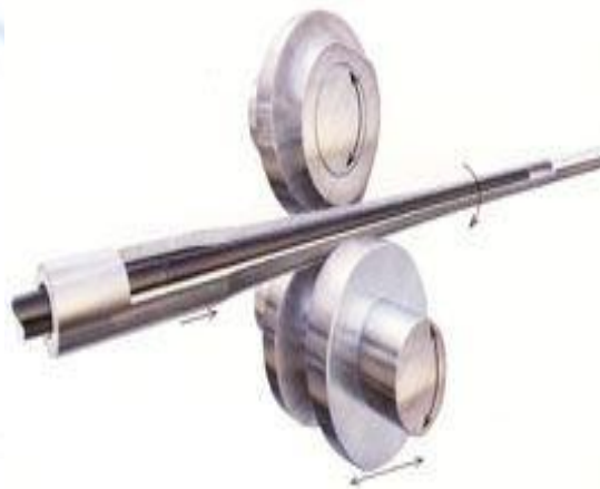
(Fig.1 Cold Pilger Process)
